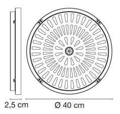
$<sup>^{\</sup>star}$  in consideration of the recycled material the measurements must be considered with a tolerance of  $\pm$  1.5%.
