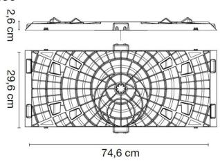
$<sup>^{\</sup>star}$  in consideration of the recycled material the measurements must be considered with a tolerance of  $\pm$  1.5%.
